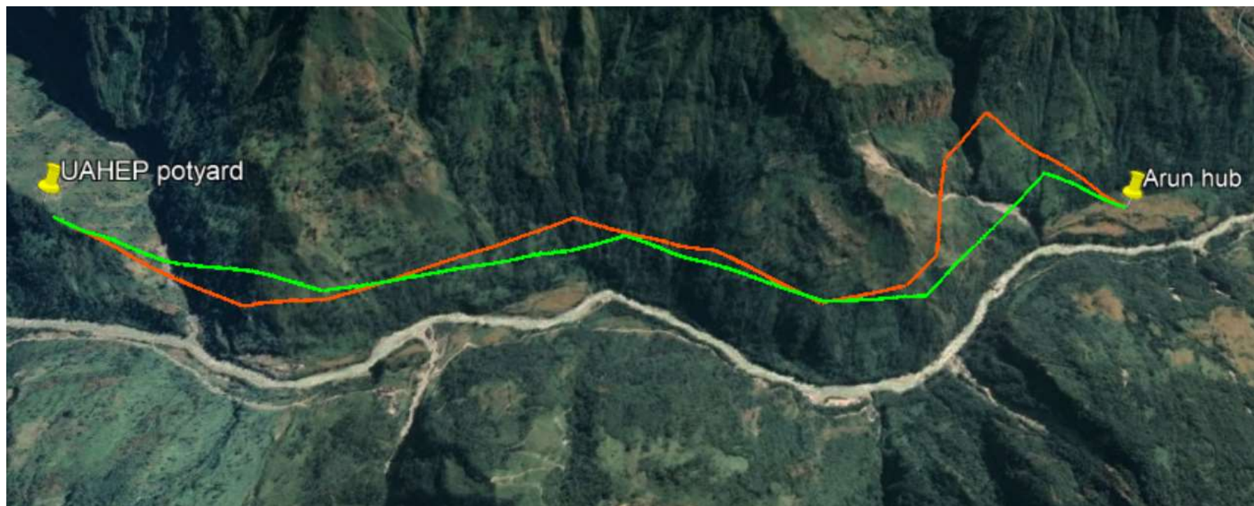
Figure 4.8: UAHEP Transmission Line Alignment Alternatives
