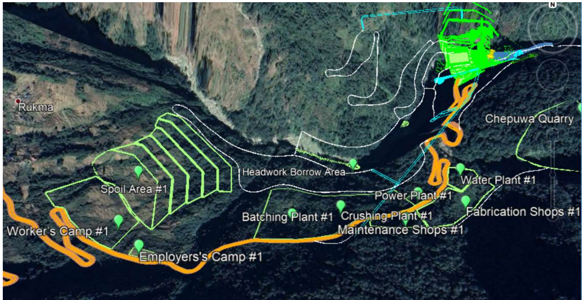
Figure 4.6: UAHEP Headworks Area Proposed Ancillary Facilities
